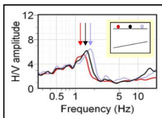
The H/V method is a non-destructive method used to map the resonance frequency of the subsurface, itself linked to the mechanical properties of the different soils and rocks present in the ground.
