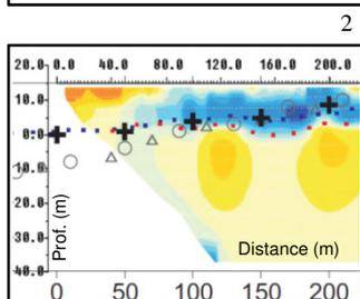
Wave propagation laws show that the ground amplifies horizontal vibrations at certain frequencies, with respect to vertical vibrations. The amplification frequency is calculated by taking the ratio of the spectra of the horizontal (H) and vertical (V) components.
