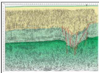
The method of seismic reflection allows the structure of the subsurface to be determined by analysing the "reflectors" vertically from the point of origin of the waves.
